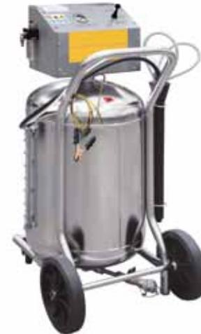
**AIR OPERATED FUEL EXTRACTOR/TRANSFER KIT WITH 100ℓ STAINLESS STEEL TANK**
